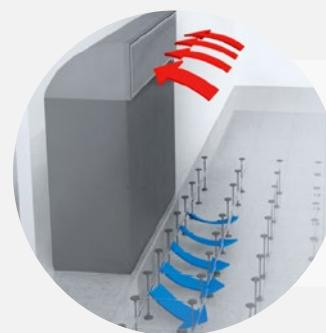
Airflow: UNDER, air discharged from the bottom and air intake from the top-rear
